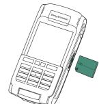
Note Insert the Memory Stick correctly to avoid damage to your P910i or the Memory Stick.
